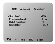
ADR radio programmes are currently radiated only from the Astra satellites in the lower frequency band (low band). The above setting is already set up accordingly. If you want to switch off the automatic search run, set the "Search run" menu entry to "OFF".
